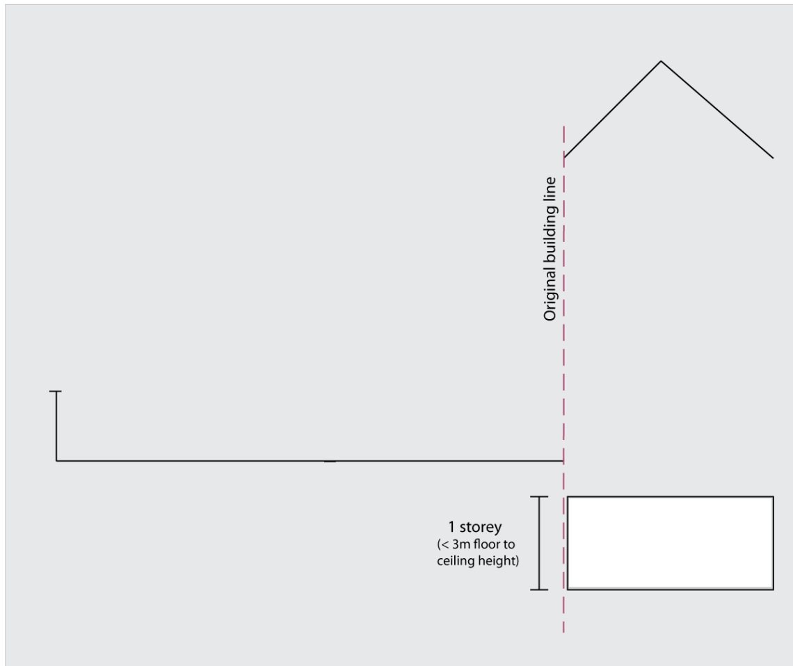
Figure 6: Maximum 1 storey depth, with floor to ceiling height no greater than 3m.
